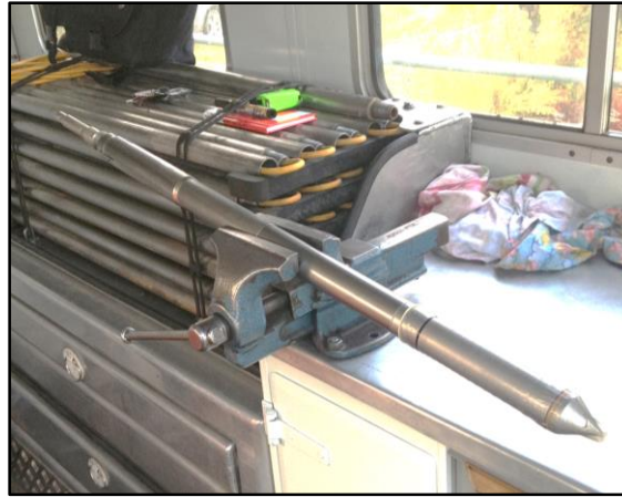
Standard Seismic CPT Cone
