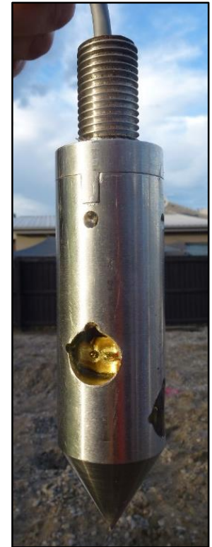
Custom Built Cones: 3 x orthogonal geophones 1 x triaxial MEMS accelerometer
