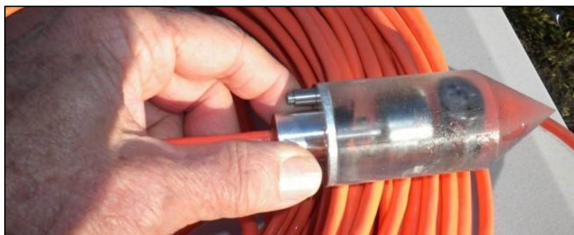
Figure 8. Ground motion sensor with two 28-Hz geophones.
