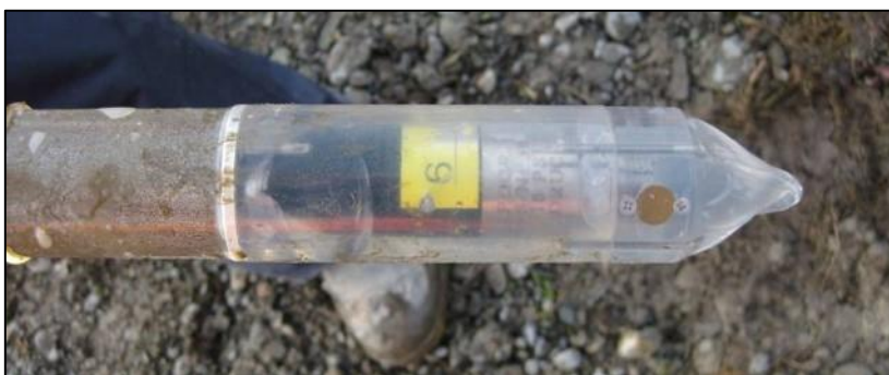
Figure 9. GE Druck PDCR 1830 Pore Pressure Transducer encased in a polycarbonate housing.
