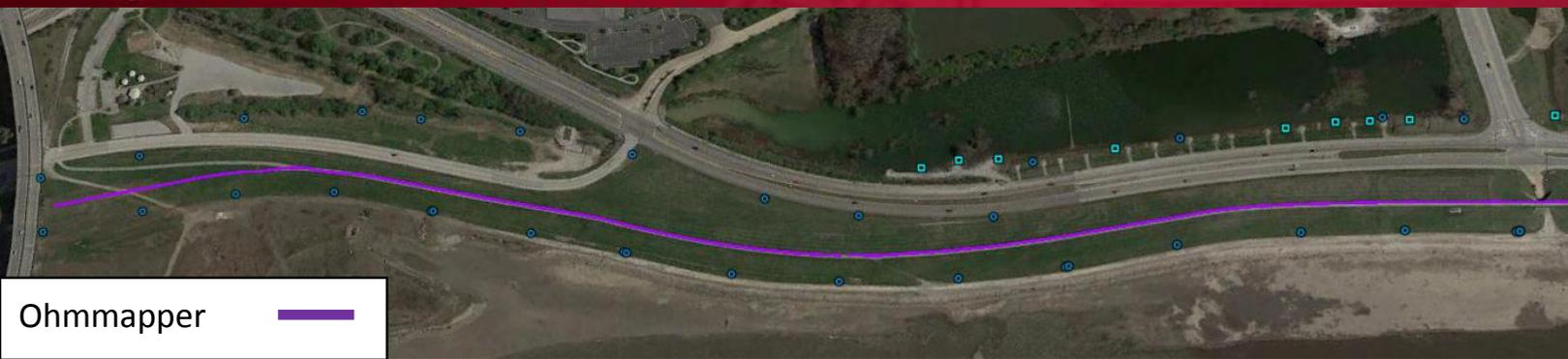
Four separate passes along Levee to obtain full Apparent Resistivity
