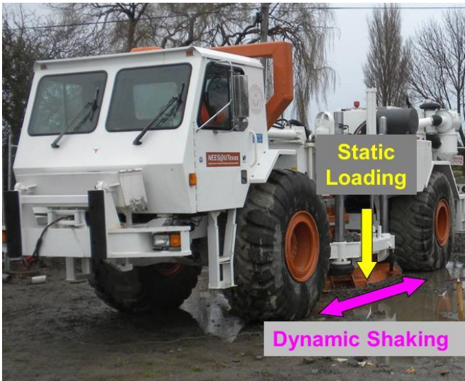
(b) Staged, Horizontal Shaking with T - Rex
