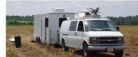
Instrumentation Van & Trailer - A customized Chevrolet cargo van provides an air-conditioned workspace - A 8 ft by 16 ft cargo trailer provides additional working and storage space
