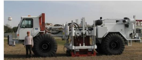
Liquidator (Low Frequency Shaker) - Off-road truck; - 32 ft long, 8 ft wide, weight = 72,000 lbs - Two vibrational orientations - One day shop transformation of shaking orientation - Shear mode Peak Force = 20,000 lbs - Vertical mode Peak Force = 20,000 lbs
