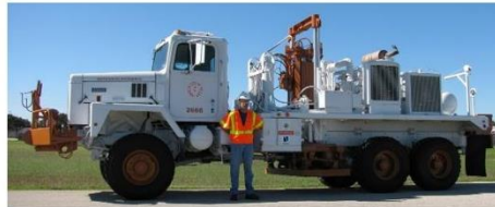
Raptor (Mid-Size Shaker) - Highway legal truck - 32 ft long, 8 ft wide, weight = 41,200 lbs - Vertical mode Peak Force = 27,000 lbs
