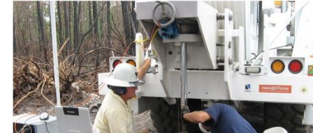
Hydraulic Cylinder with Adjustable Platform - Mounted at the rear of T-Rex - Platform for installing and retrieving liquefaction, CPT, and seismic CPT sensors
