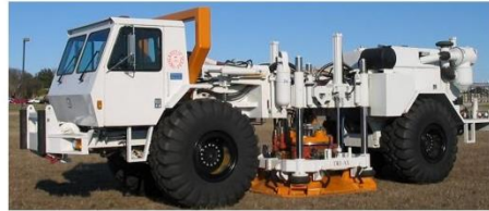
T-Rex (Tri-axial Shaker) - Off-road buggy; - 32 ft long, 8 ft wide, weight = 64,000 lbs - Three vibrational orientations - Push-button transformation of shaking orientation - Shear mode Peak Force = 30,000 lbs - Vertical mode Peak Force = 60,000 lbs
