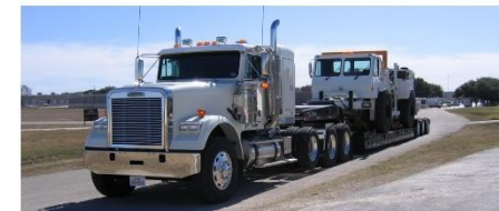
Big-Rig - 26 wheeler tractor-trailer rig for shipping T-Rex, Liquidator, and Rattler - Overweight permit required
