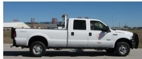
Fuel-Supply Truck - Carries diesel fuel for T-Rex, Liquidator, and Rattler in the field - provides a working platform for maintenance and CPT tests
