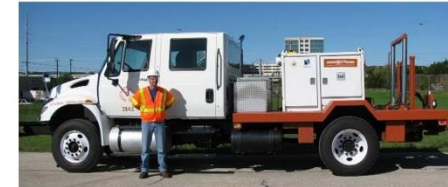
Thumper (Urban Shaker) - Built on a International 4300 truck; - 27 ft long, 8.5 ft wide, weight = 24,800 lbs - Three vibrational orientations - Four hours field transformation of shaking orientation - Shear mode Peak Force = 6,000 lbs - Vertical mode Peak Force = 6,000 lbs
