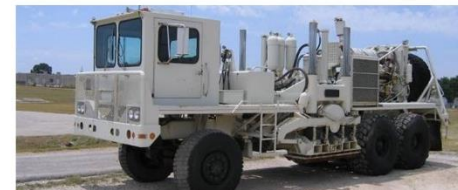
Rattler (Horizontal Shaker) - Off-road truck; - 29 ft long, 8.5 ft wide, weight = 54,500 lbs - Shear mode Peak Force = 30,000 lbs
