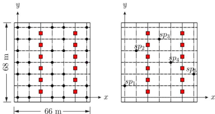
(b) Experiment layout; sensors (dots) - sources (squares); control sensors
