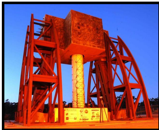
Shake table testing at UC San Diego
