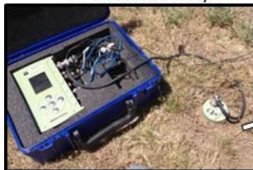
3D Seismometers In Circular Arrays
