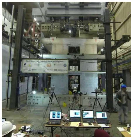
Hybrid testing at Lehigh
