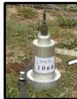
3D Seismometers In Circular Arrays
