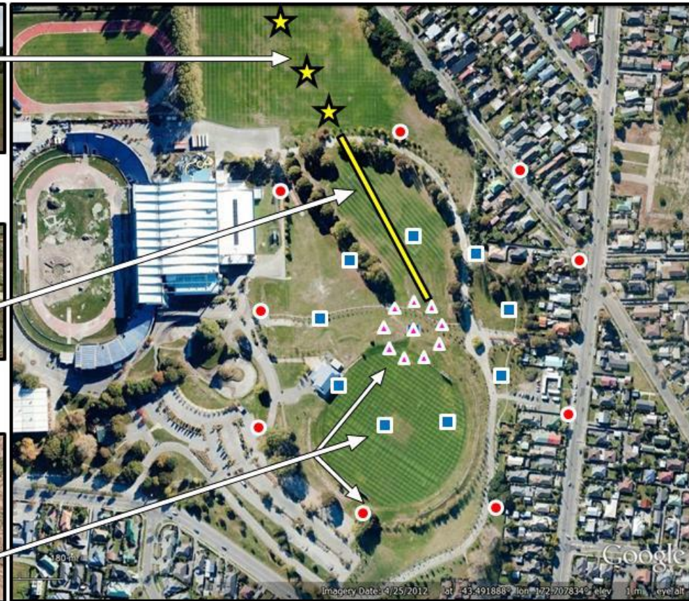
3D Seismometers In Circular Arrays
