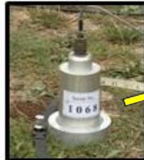
3D Seismometers In Circular Arrays
