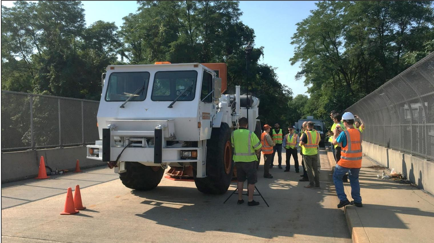
Preparing to dynamically load a two-span bridge over Interstate Highway I-195 in Trenton, NJ. Bridge deck was loaded longitudinally and laterally and the motions were large and easily seen. Shared-use project was performed for Professors Nenad Gucunski, Franke Moon, and John DeVitis from Rutgers University
